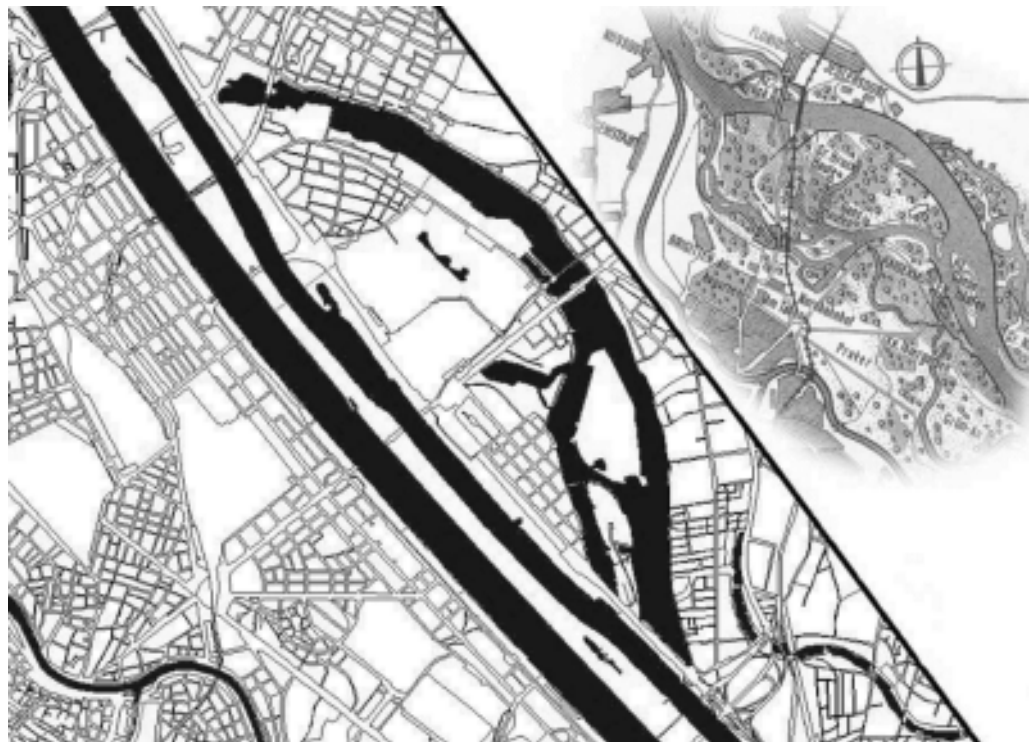
Fig. 1. Map showing the original water way of the Danube in the mid-19th century in Vienna (upper right) and the situation as it appears in 2004.
